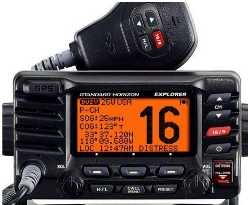
2) Lift the RED distress button cover on the lower right. Underneath is a red button. Press the button and hold it for 4-5 seconds and then release the button. In a few seconds, there will be a loud alarm coming from the radio's speaker. Touching any button on the radio will stop the alarm.
